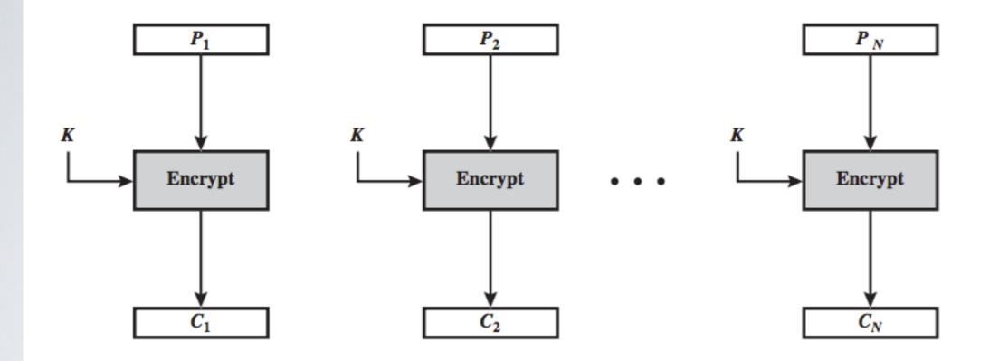
Each plaintext block is encrypted independently with the key
