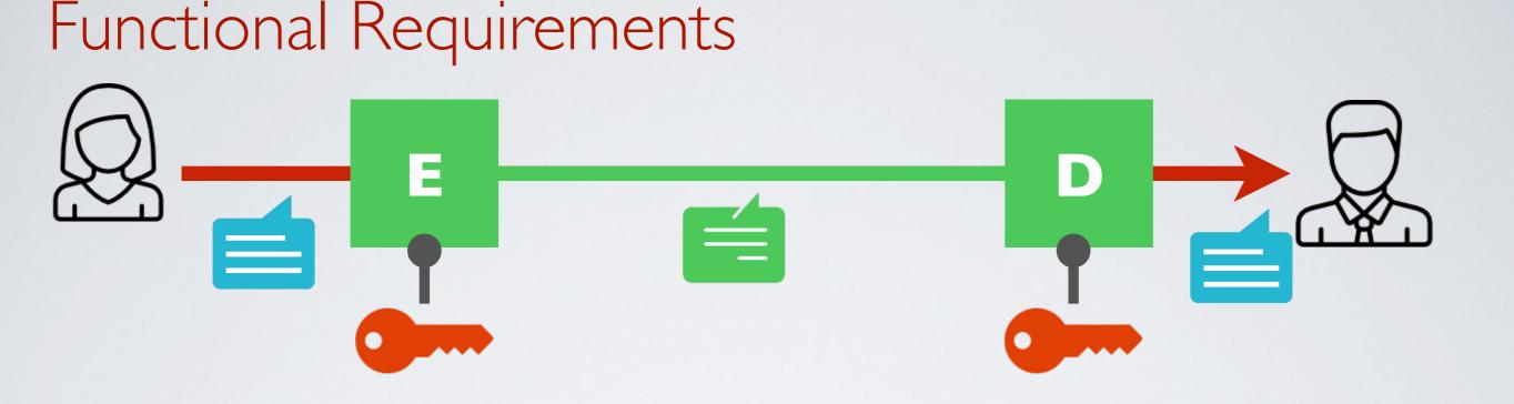
The same key k is used for encryption E and decryption D
